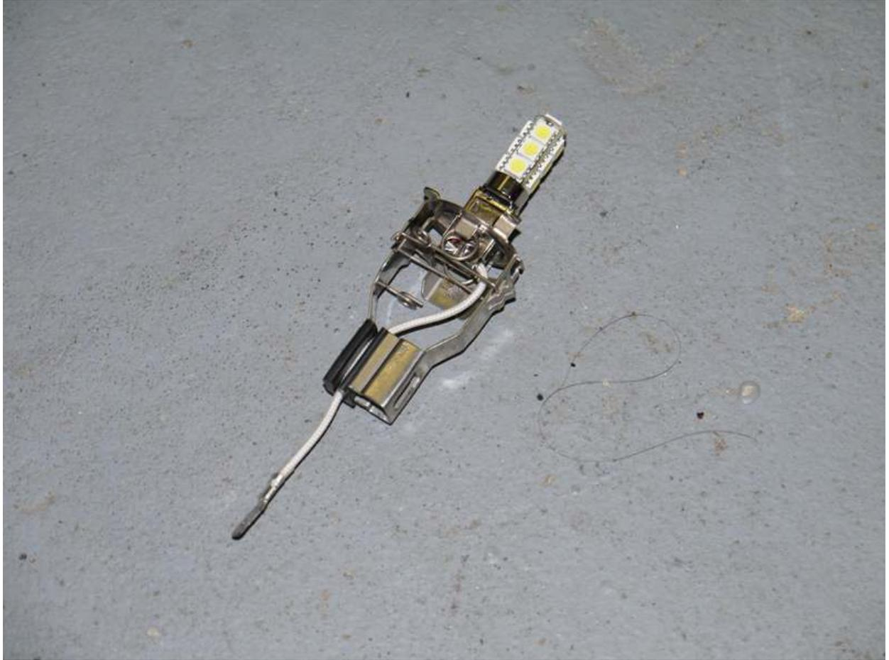
**Step 5-** Connect the wires to the led bulb and carrier, you must reverse the wires in order for the led bulb to work, led is reverse polarity. On the factory bulb the red wire was connected to the lead of the bulb it must now be connected to the ground on the carrier, once again the red wire to the ground of the carrier, the black wire must be connected to the lead of the led bulb.
