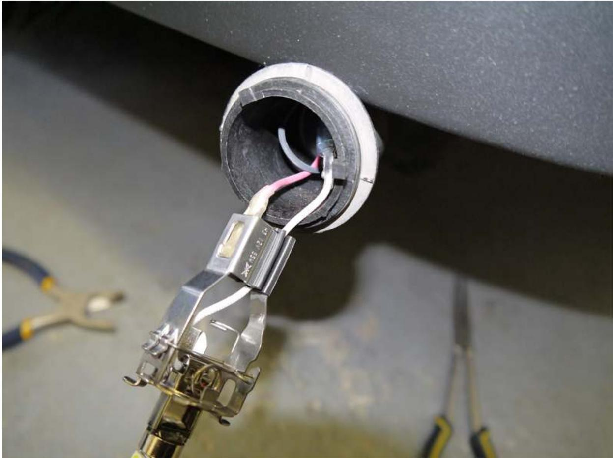
**Step 6-** Install the carrier inside the fog light housing , this requires patience as there's not much room to work with, remember that you had to turn the carrier to remove it, the same applies to install it. Once the carrier is secured install the cover. Repeat for the other side.
