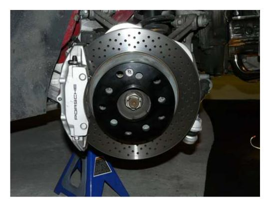
**Step 4** – Install your Wheel, make sure it clears the inside of the wheel and that it doesn't rub against anything, torque to manufacturer torque specifications normally 130 Nm (96 ft. lbs.). Do not use any power tools to tighten the wheels.
