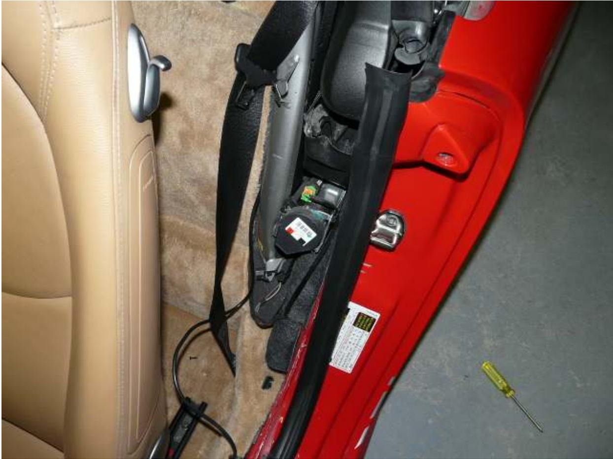
Remove trunk trim with allen key, look carefully there's 2 little caps that need to be removed on the sides, this will enable you to insert the allen key, simply unscrew a few turns do not remove the screws, once the screws are loose pull the trim up , remove electric connector.
