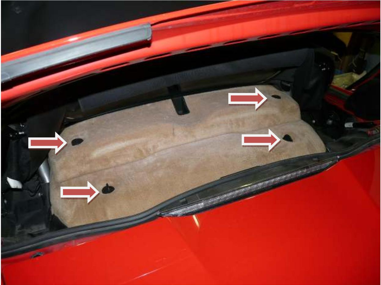
**Step 3-** Remove the engine cover by removing the 6 torx screws.
