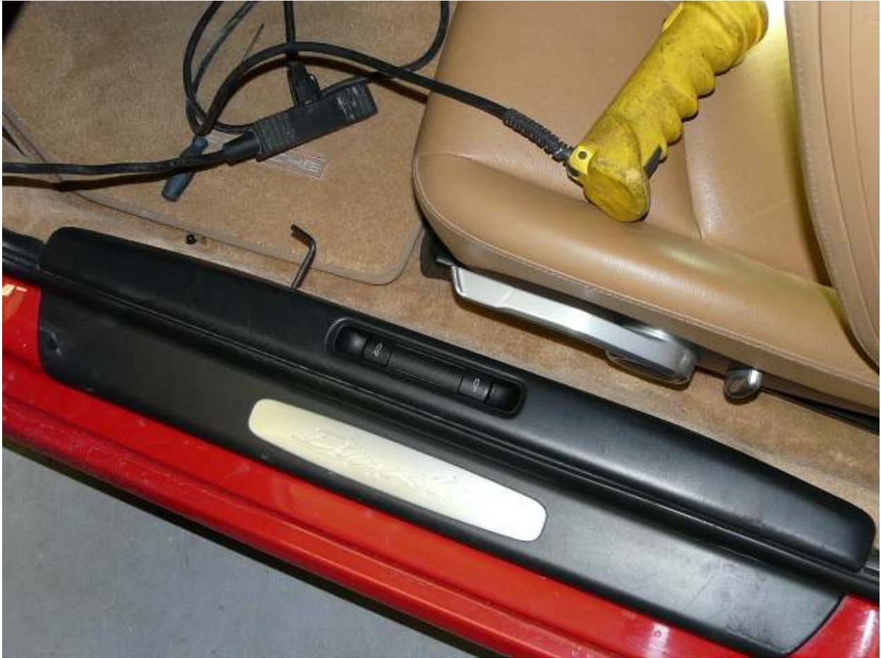
Remove the 3 screws on the fuse box trim , pull out the fuse box trim.
