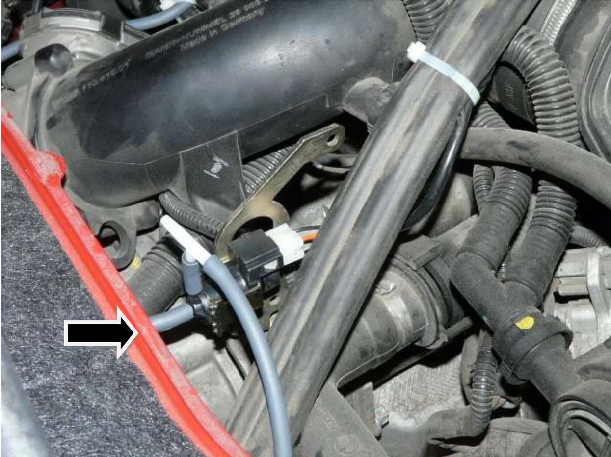
Now plug the two foot hose to the white valve, if the 2 foot hose is too long cut it accordingly.
