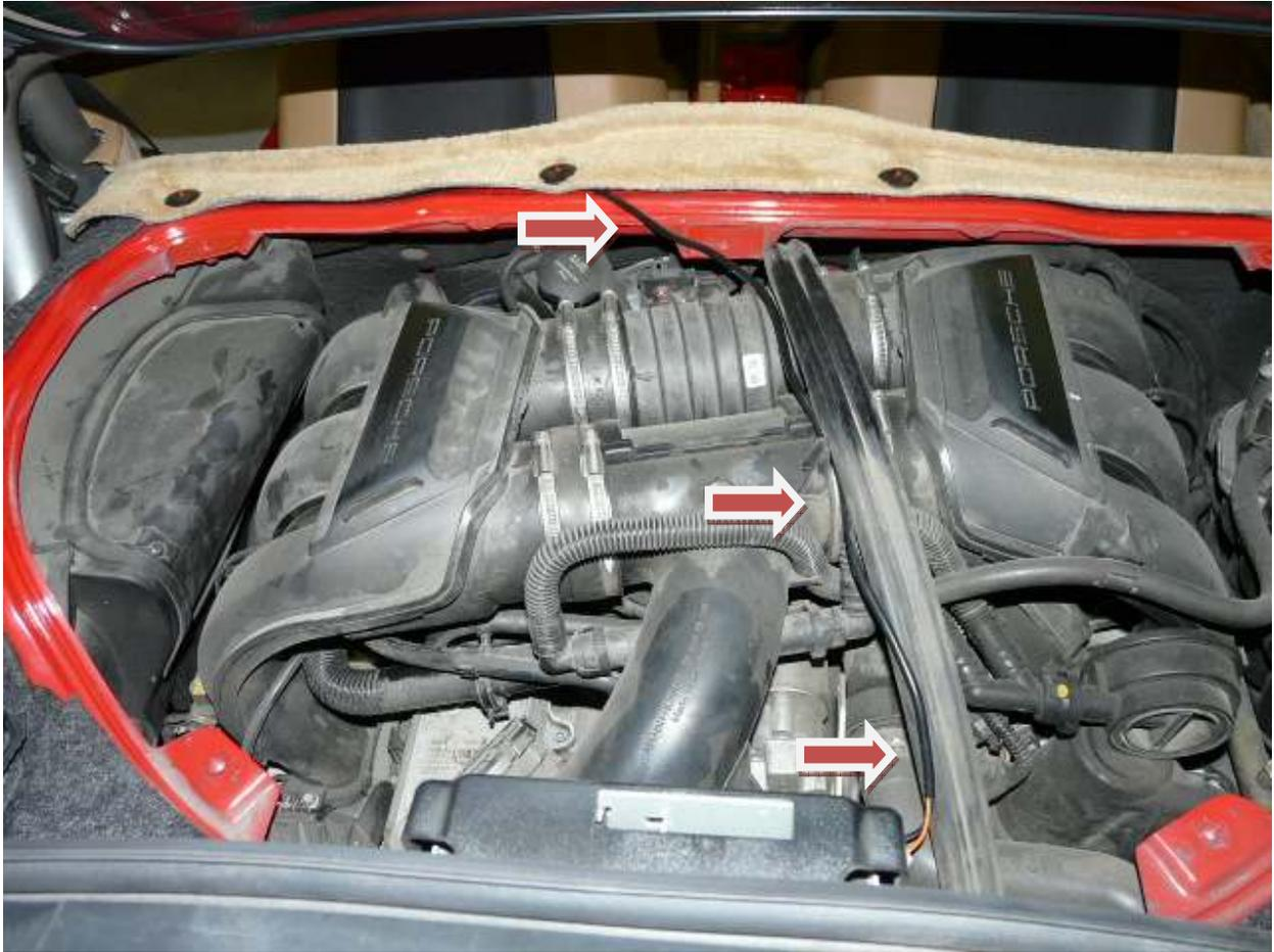
Remove roll cage trim, there's a small Philips screw on the side of it, you need to look carefully to spot it, once removed pull the trim up and it will come out.
