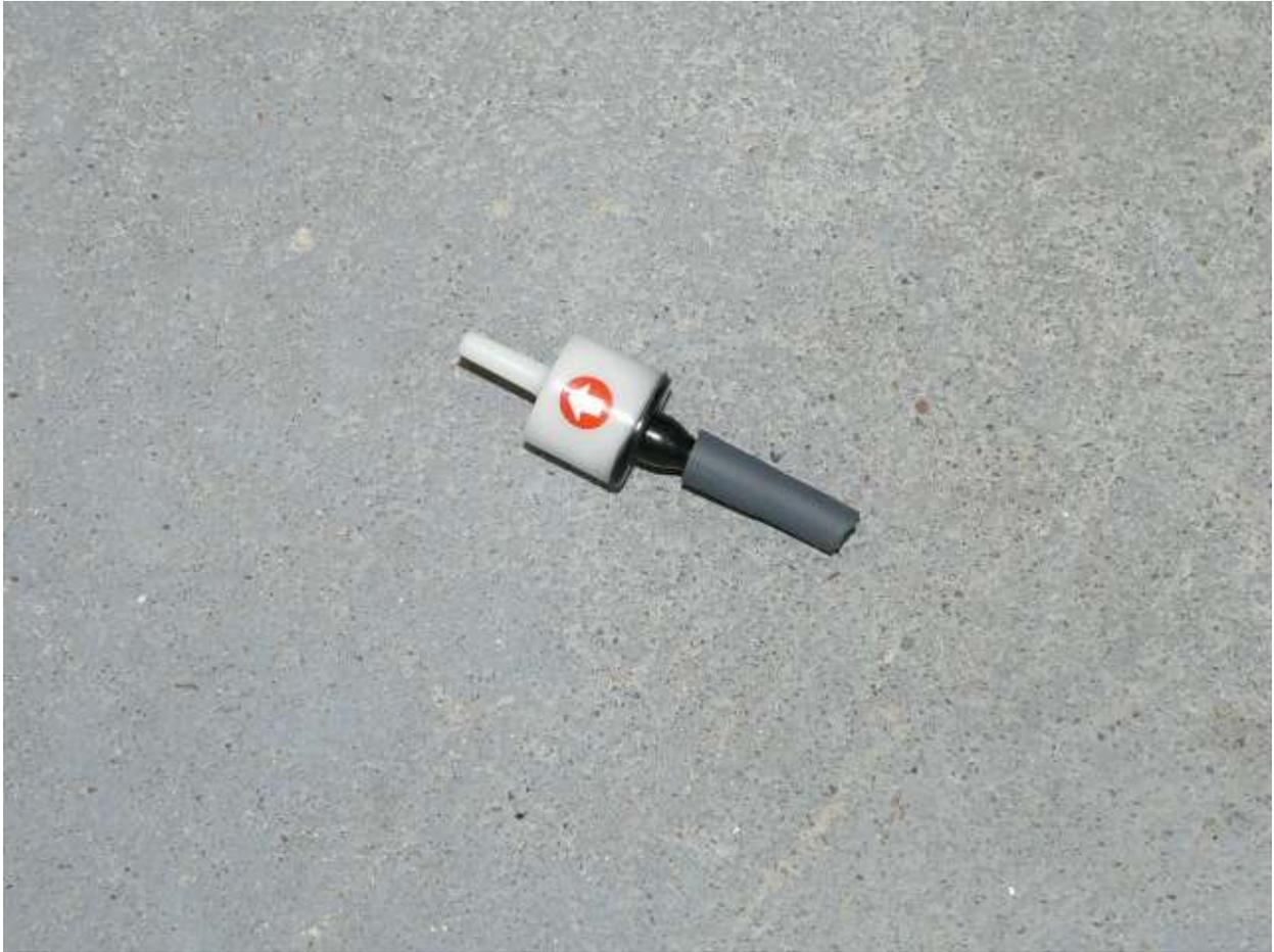
**Step 9-** Install the small white valve with the arrow on it , on the bottom nipple of the solenoid valve , insert the vacuum line in the bottom nipple.
