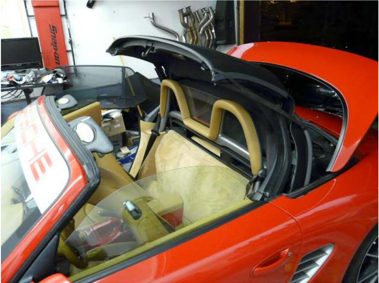
**Step 2-** Remove the rear storage box by unlocking the two lock pins that retain the storage box in place, pull out the storage box . Once removed , remove the 2 lock pins for the carpet trim and pull out the carpet trim.
