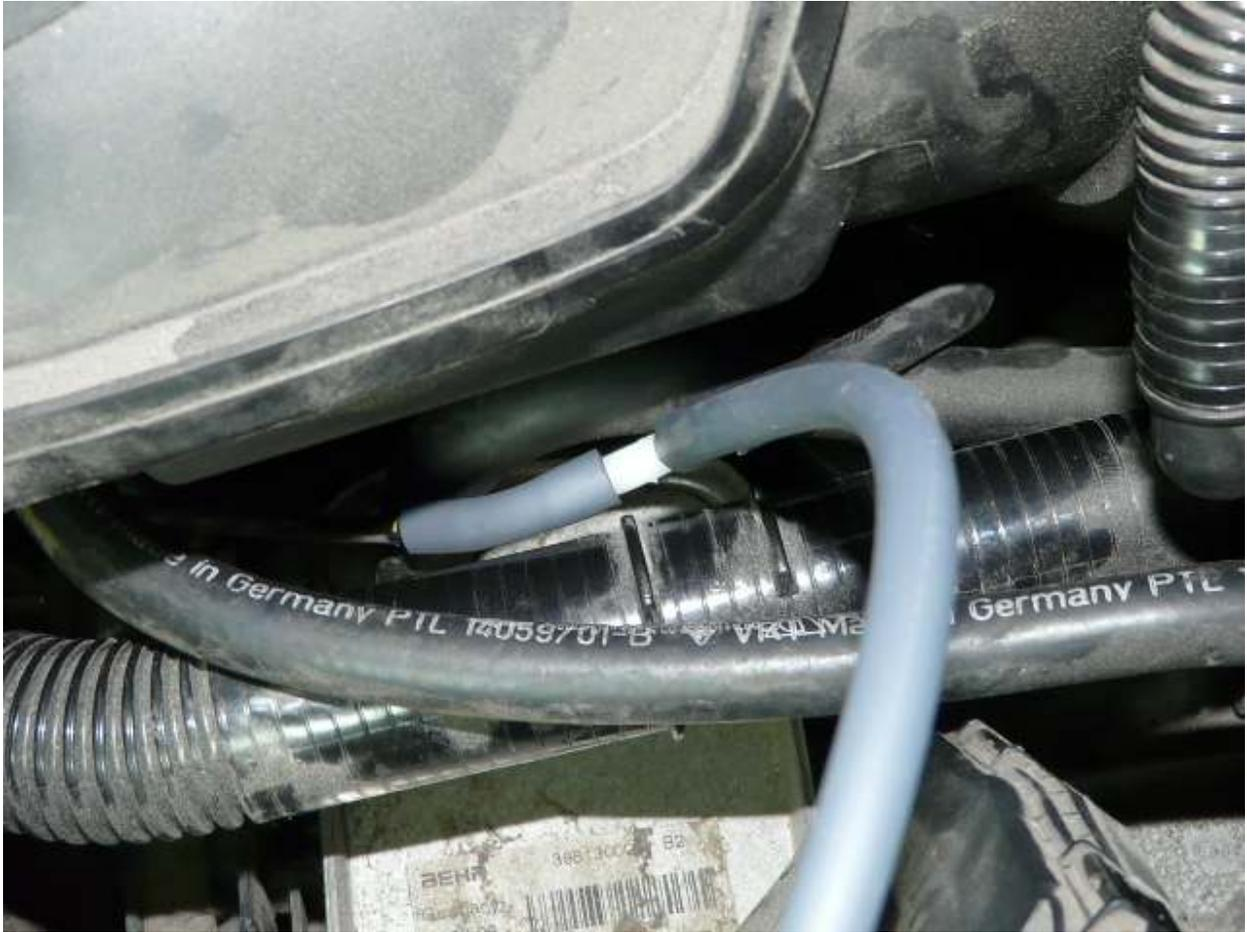
**Step 8-** Install the small white valve with the arrow on it , cut approx 1 inch rubber hose and install it on the valve as shown .
