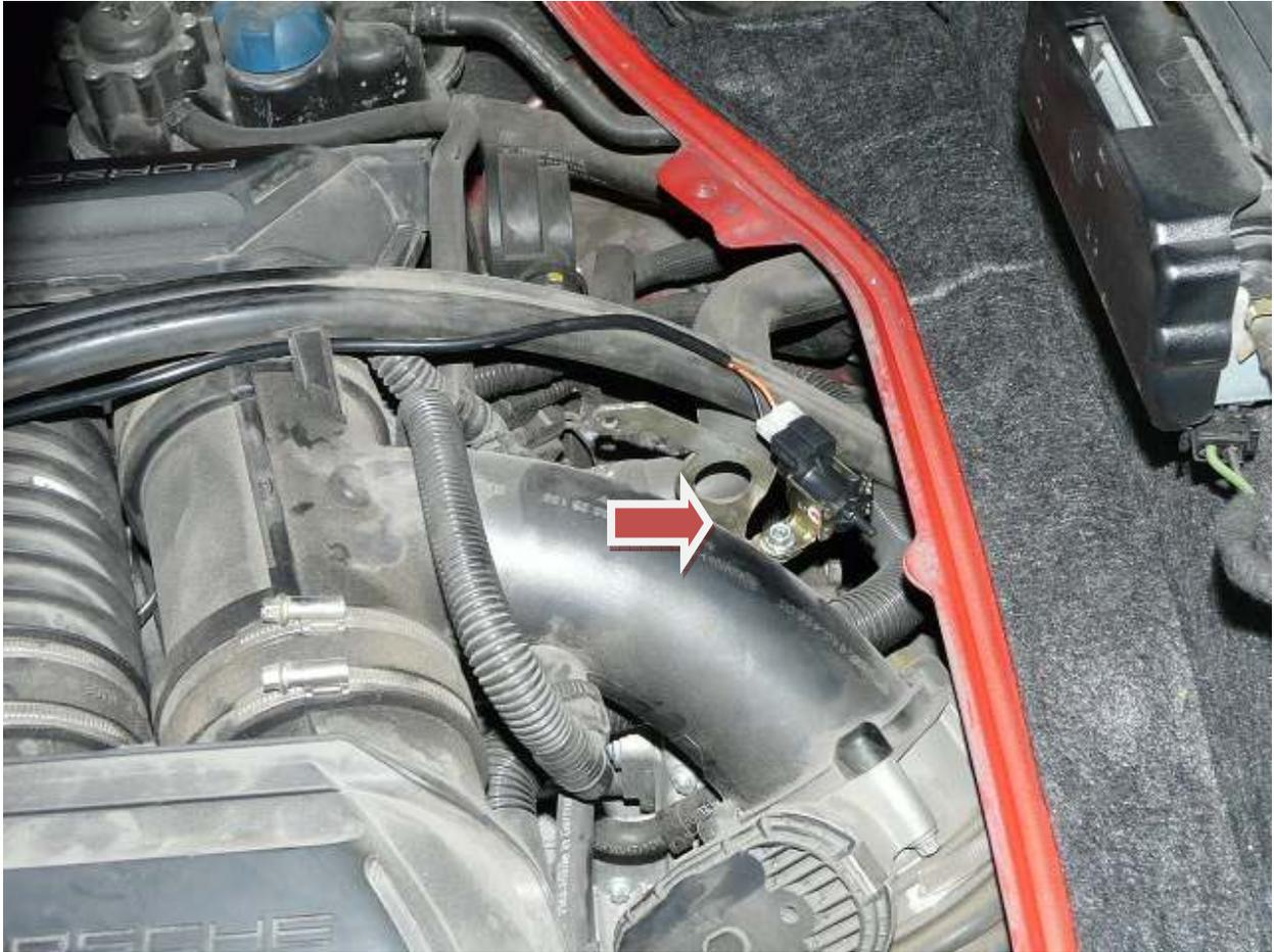
**Step 5-** now we will need to route the electrical wiring harness from the solenoid all the way to the interior cabin of the car, I slipped the wiring under the carpet trim and brought it forward , the wiring will be routed behind the roll cage trim and under the door sill trim inside the car to finally bring it close to the fuse box.
