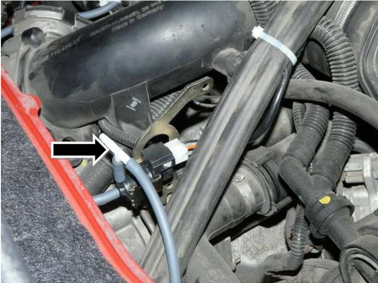
**Step 11-** You will need to route the vacuum lines from the mufflers all the way to the t-pipe, secure lines with Tie-Wraps.
