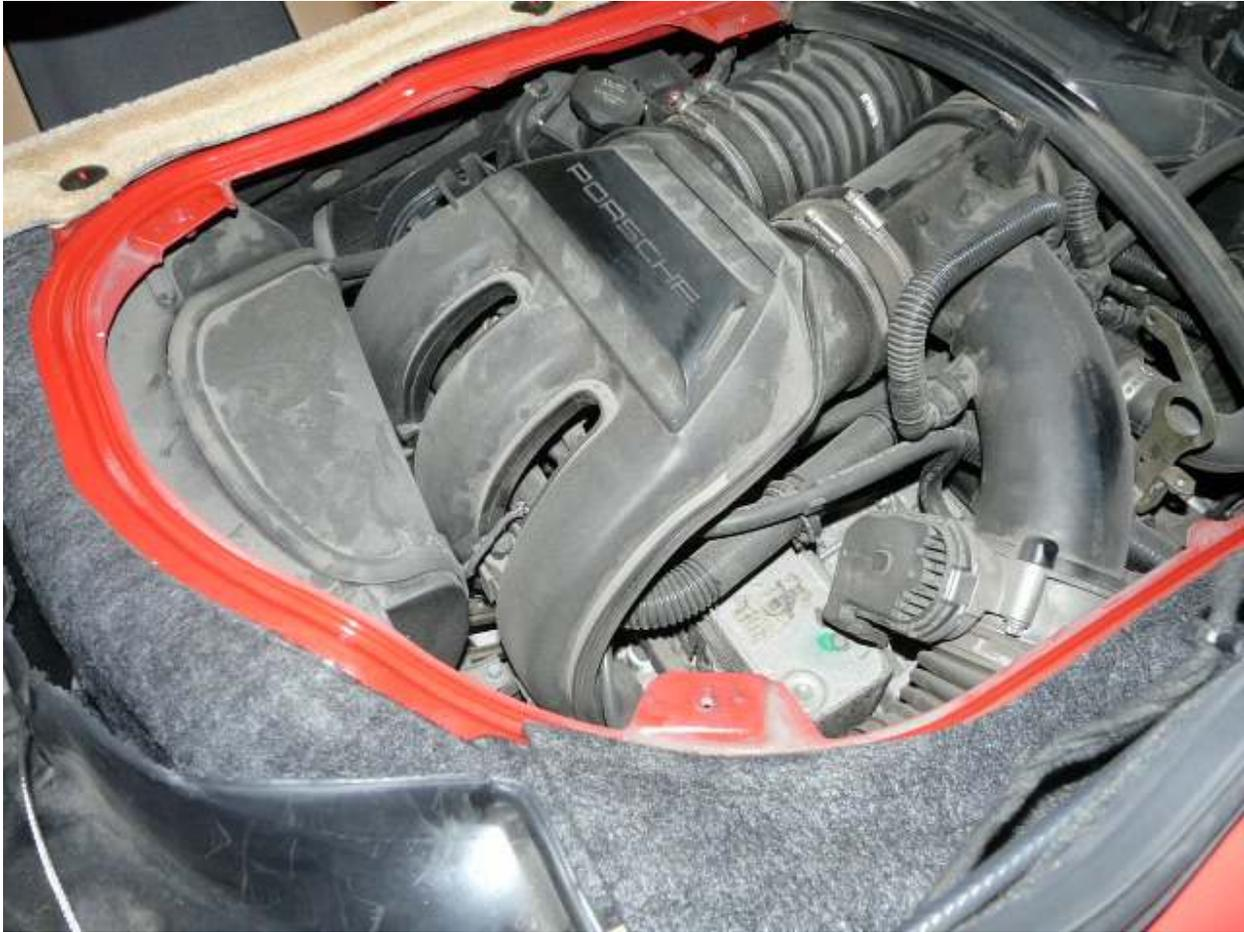
**Step 4-** The first thing we need to do is to find a good location for the solenoid valve, you can pretty much use your imagination but I have found a nice spot right next to the throttle body there's a engine hook, see the picture below. You can secure it with the included bolt.
