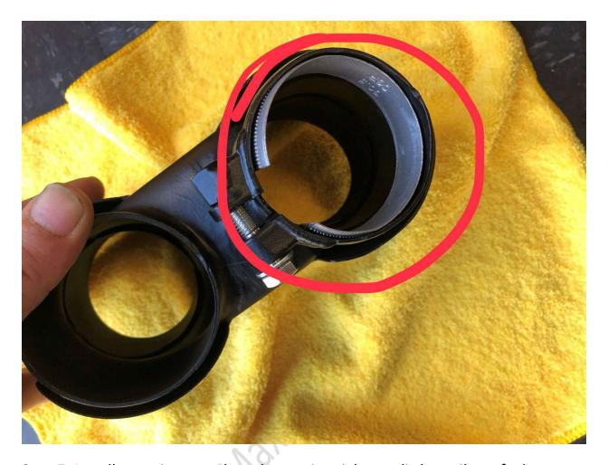
**Step 5-** Install your tips over the exhaust pipe tighten a little until you feel some resistance in moving the tip, now adjust to your liking left to right and back or forward, once you have achieved your desired position tighten the 13mm bolt until the tip is tight and no longer moves don't overtighen just toghten until tip no longer moves.
