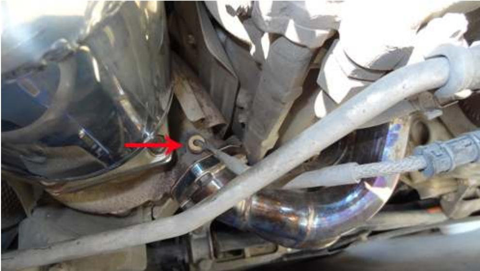
Step 7- Install the catalytic converter with the supplied gasket, make sure you position the turbo heat shield correctly , tighten all 4 turbo bolts. Remember to tighten the small exhaust port bolt on the side of the catalytic converter. Re-clip your O2 sensor wiring and connect the O2 sensor wiring connectors. Replace the air box cover.
