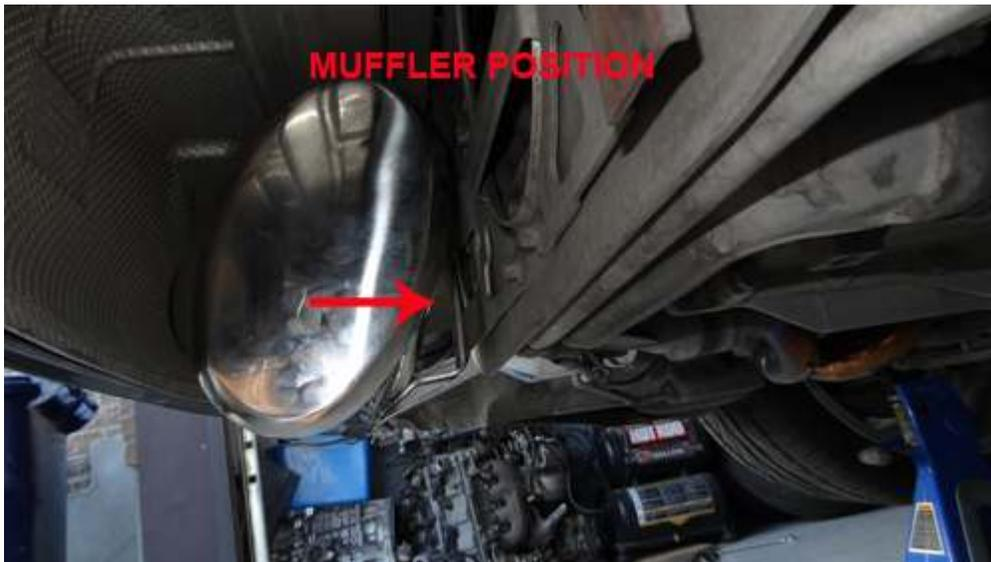
Step 10- Tighten Muffler clamps between the catalytic and the muffler, hold your muffler straight and tighten clamp, now tighten the steel belts, you will need to use an extension to reach the tightening bolt of the steel belt.
