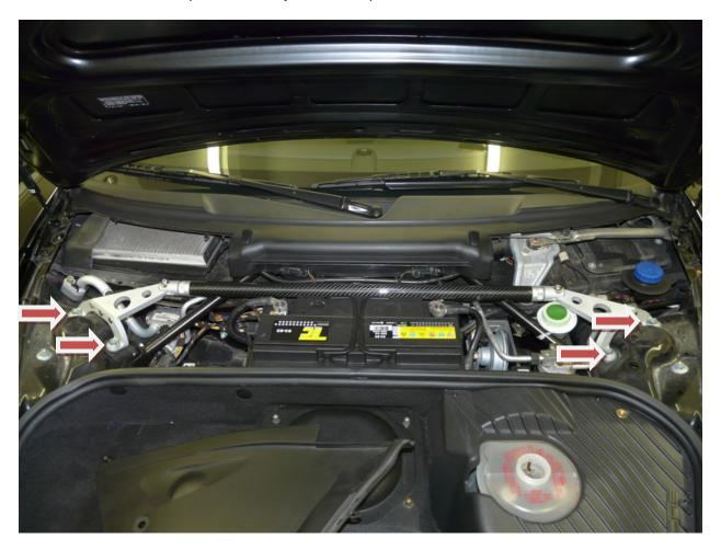
**Step 3** – Position strut behind the battery and insert arms on strut tower studs. Tighten the 2 x 13mm nuts over the aluminum strut bar arms, tighten just enough, don't over tighten as you could break the studs.
