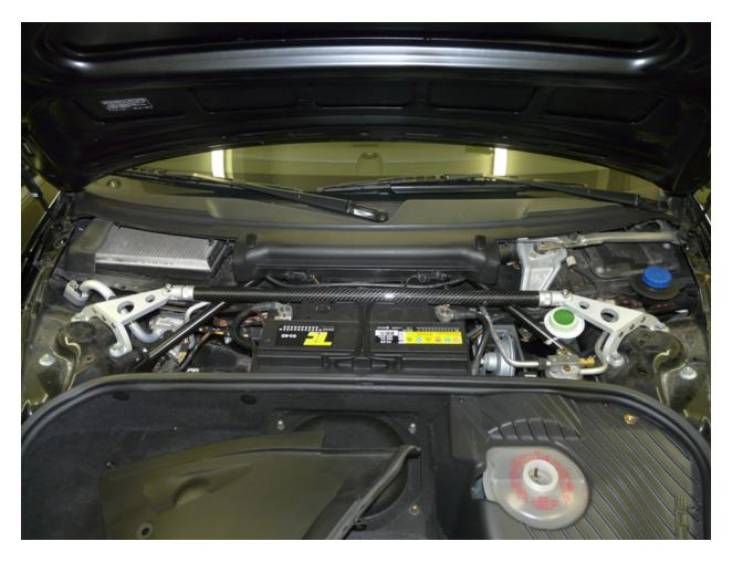
**Step 4** – Once installed you must tighten all the screws on the strut brace.
