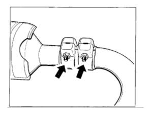
**Step 11-** Start by tightening the double clamps as tight as possible excessive force is needed to tighten them properly, tighten the muffler clamps.
