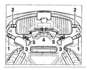
Step 5- Remove the two top hexagon collar nuts M8 (a/f 13) on the transmission bracket -arrows-
