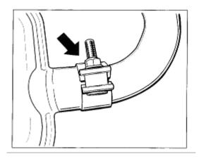
**Step 4** – Detach the two retaining plates on the catalytic converters left and right -3- and the bottom holder on the transmission bracket -4-. To do this, unscrew the four hexagon-head bolts M8 and two hexagon nuts M8 and remove the retaining plates and threaded plate respectively. For better access to the top collar nuts, the holder can be removed by undoing the hexagon nuts M8 -5-.
