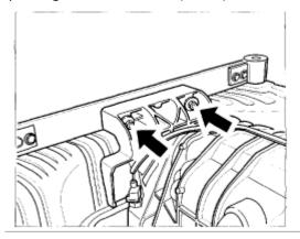
**Step 6-** Push rear muffler towards bumper and press the retaining plate to the the rear between the studs **-arrow-** to guide the studs out of the transmission bracket. Carefully tilt the rear muffler downwards and with the help of a second person remove it past the rear apron.
