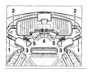
**Step 1-** Remove exhaust pipes at the sides. To do this, open the double clamping sleeves by undoing the hexagon nuts M8 and moving them towards the catalytic converters. If necessary, prise the clamps apart and then move them. If there is corrosion, removing the exhaust pipes and clamps is made easier by heating.
