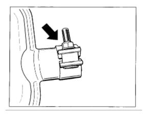
**Step 10-** install U-Bend Pipes inside the muffler ends and align them with your cat-pipes and slide over the double clamps
