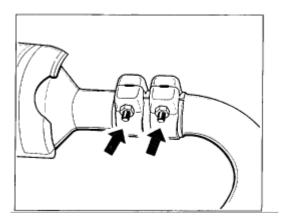
**Step 3-** Open the clamp on the rear muffler connection by undoing the hexagon nut and push it onto the exhaust pipe. Pull the exhaust pipe with twisting movements out of the connection and remove it.
