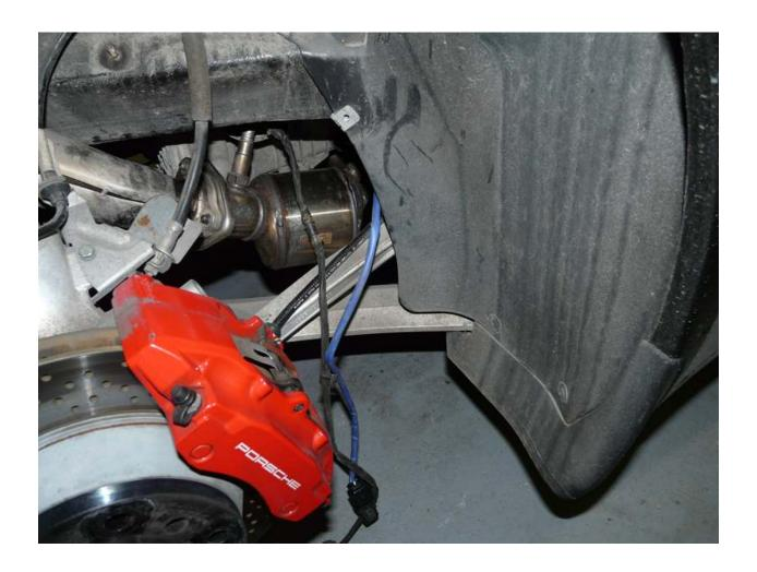
**Step 3** – Inspect the factory steel gaskets, we recommend that you re-use the factory gaskets they are made out of steel and are superior gaskets. You will need to remove the two oxygen sensors and install them on the new racing header, remember to install them in the same position, the blue wired sensor is the first sensor (upstream sensor) black sensor is the downstream (2<sup>nd</sup> sensor).
