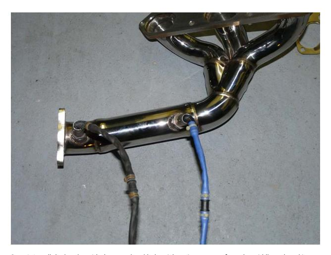
Step 4- Install the header with the same head bolts, tighten in sequence from the middle and working your way out and torque to specs First stage to 25 Nm (18 ftlb.).
