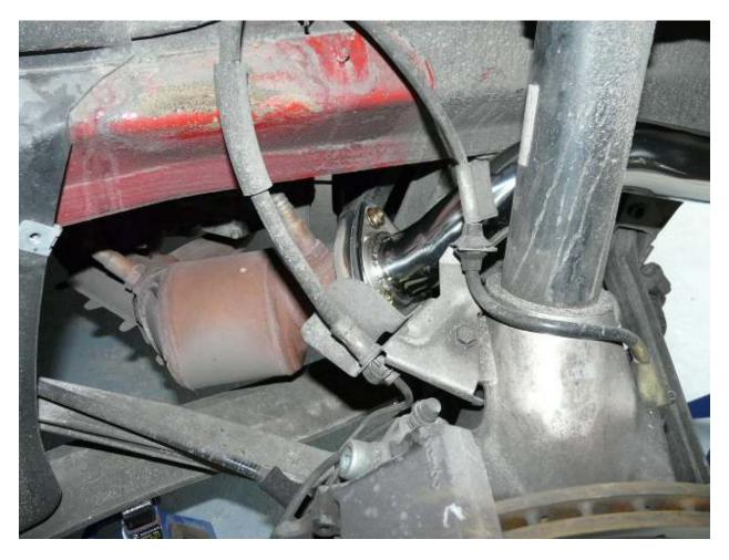
**Step 8-** Install the Muffler supports, please see pictures below on how the supports should be assembled and installed.
