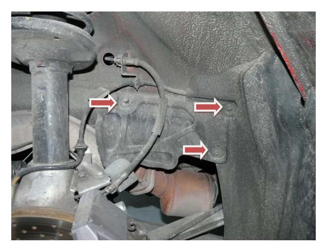
**Step 2-** Using a few extensions with a ratchet and 13mm socket remove the 3 bolts that connect the mufflers to the headers.
