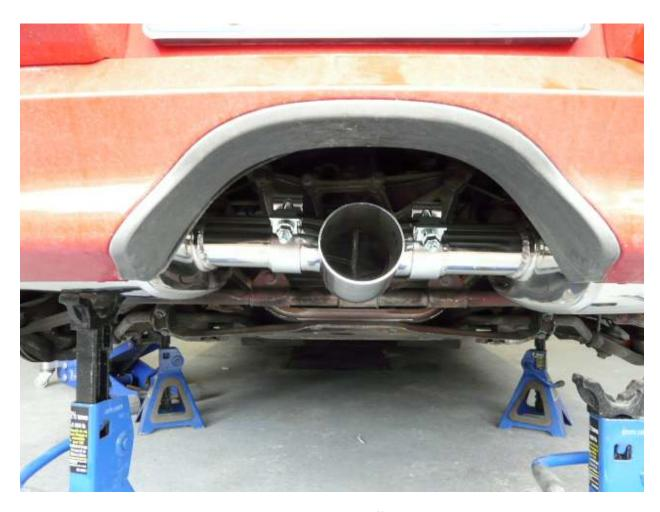
**Step 7**- Now tighten the bolts between the headers and mufflers.
