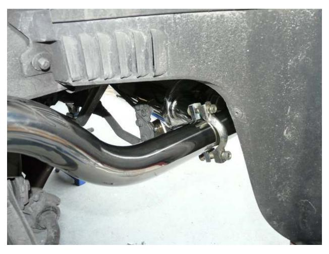
**Step 9-** Now position Y-Pipe at your desired angle , tighten both clamps and finally install the exhaust tip.
