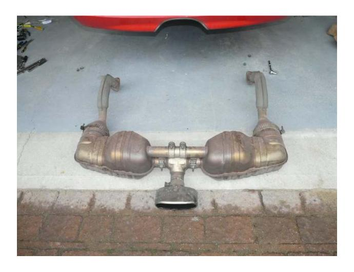
**Step 4**- You are now ready to install the NHP Exhaust. Start by installing both your gaskets on the exhaust headers.
