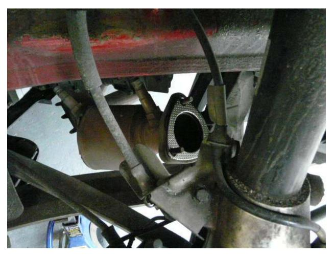
**Step 5**- Install both the left and right side mufflers without tightening any of the bolts and support your mufflers with jack stands.
