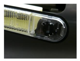
**Step 7** - You are ready to install your new 3<sup>rd</sup> brake light, simply install it in the 3<sup>rd</sup> brake light cut-out, make sure you insert the black tab on the left of your 3<sup>rd</sup> brake light behind the cut-out. Now lock the tab with a screwdriver so that the 3<sup>rd</sup> brake light is secured on the trunk lid, and install your small cover.
