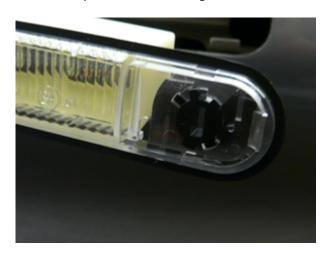
**Step 7** - You are ready to install your new 3<sup>rd</sup> brake light, on the 996 Turbo it's a tight fit, the easiest way to install it is by applying some lubrification around the gasket, the best would be water with dishwashing soap, just a small amount I mean small amount to be applied with your finger around the black gasket on the 3<sup>rd</sup> brake light, again small coating doesn't need to drip.
