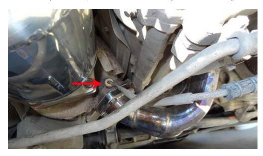
Step 7- Install the catalytic converter with the supplied gasket, make sure you position the turbo heat shield correctly, tighten all 4 turbo bolts. Remember to tighten the small exhaust port bolt on the side of the catalytic converter. Re-clip your 02 sensor wiring and connect the 02 sensor wiring connectors. Replace the air box cover.
