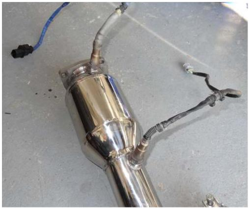
Step 6- You are now ready to install the cats, before doing so remove the exhaust temperature sensor and stash away on the side, this will make it easier to tighten the turbo flange bolts.
