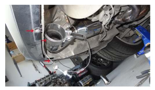
Step-9 Install the muffler cans, the belts are shaped like the muffler shape meaning belts are pre-bent please familiarise yourself prior to installing the muffler cans.
