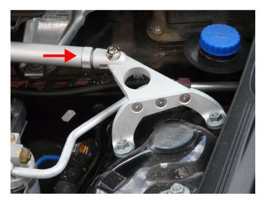
**Step 6-** You should now tighten the Allen Screw and Bolt that connects the arms to the bar.
