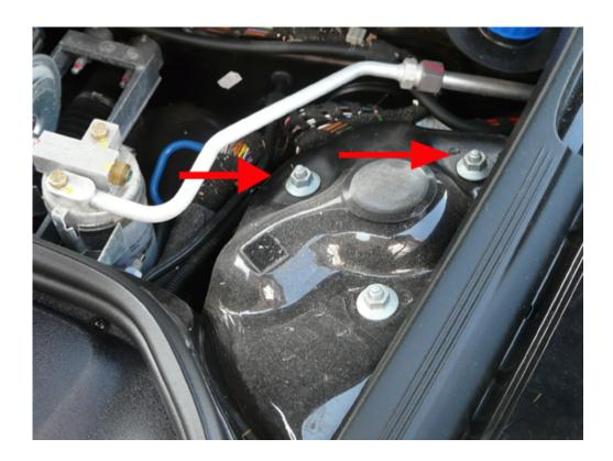
**Step 4** – Mount the Strut Brace by passing it behind the battery , mount each arm of the strut towers , if your short a few milimeters or centimetres simply rotate the arms to give it more length, once positioned you can tighten the strut brace to the strut tower with the 2 nuts previously removed on each strut tower.
