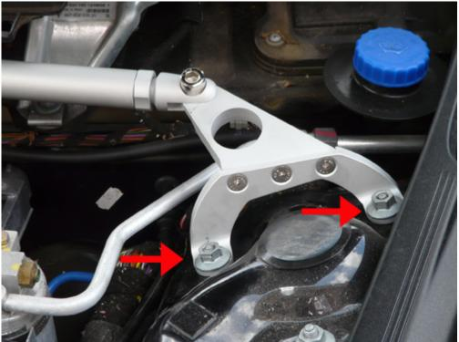
**Step 5-** You should now tighten the length adjustment bolt by hand by tightening it on the inner side of the strut brace.
