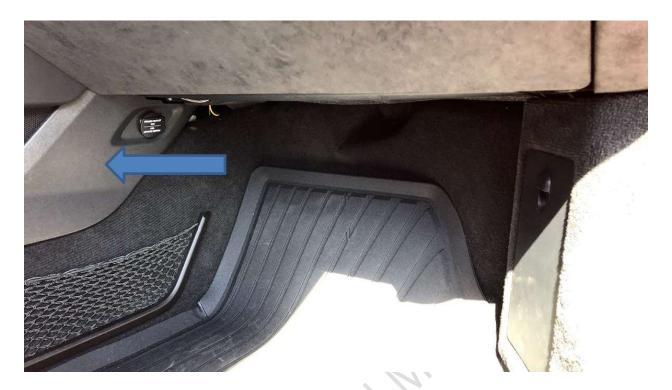
Remove the fuse box cover and trim. Pull the fuse box trim towards the center console and then pull back towards the rear of the car the trim ill come off.
