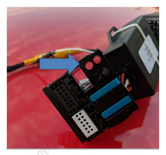
**Step 6-** Install the PCM Adapter to the Porsche PCM Harness basically the adapter will now fit between the Porsche factory PCM harness and the PCM Radio, make sure the connector is locked. Don't install the radio yet.
