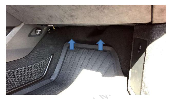
Remove the door sill trim, this trim is clipped insert pry tool and pry it out.
