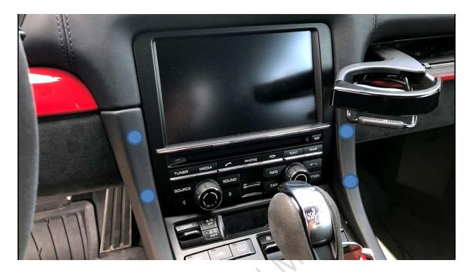
**Step 4-** Disconnect the Black Connector from the PCM, disconnect the various antenna cables (up to 4 of them) and set the PCM on the side.
