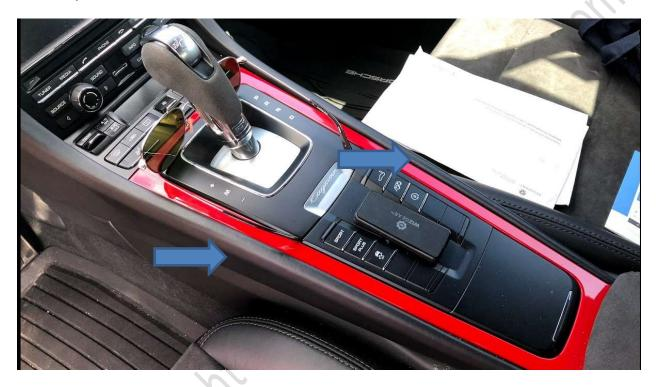
**Step 3-** We recommend you use some shop rags or towels and place these on your center console and over your shift knob to avoid any damage or scratches. Remove all 4 screws and pull out the PCM. See blue dots shows where screws are located behind the trims.
