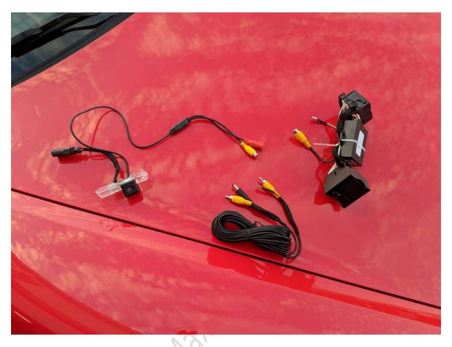
**LEFT:** CAMERA WITH BUILT-IN LICENSE PLATE LIGHT - **MIDDLE:** VIDEO AND POWER CABLE - **RIGHT:** PCM HARNESS WITH PCM EMULATOR
