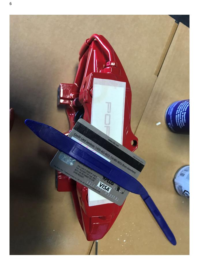
**Step 2**- Now make a cardboard cutout, this way when you spray paint the stencil it will not overspray on the caliper.
