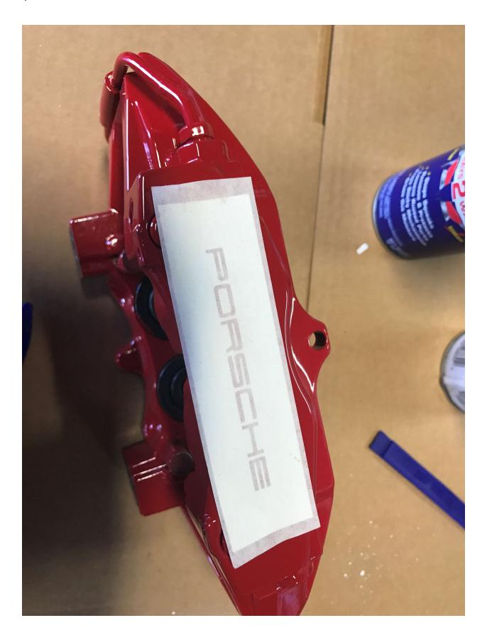
c) Press on the stencil so that it sticks properly, now use a credit card and at And the Read Hotors Ports Com gently pass over the stencil a few times.
