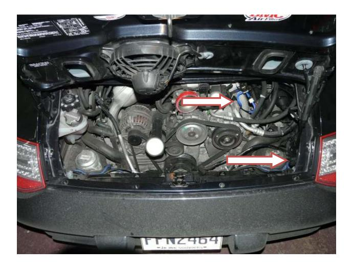
**Step 2-** Ok let's start the installation. FOR 996 Start by removing the Air Cleaner Box assembly, loosen up the intake boot clamp on the throttle body, remove the center bolt (right in front of the hood latch), disconnect Mass Air Flow connector, unclip mass Air Flow wiring from the air Box, slowly pull out the air box assembly.
