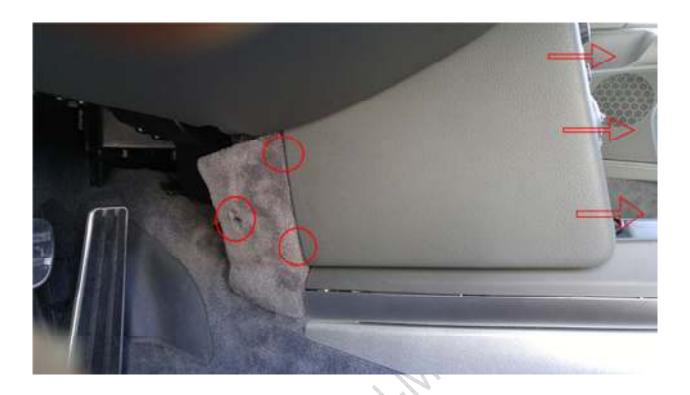
**Step 2-** Push on the gold clips on both sides and push the HVAC Unit out, disconnect the electrical connectors.
