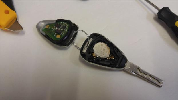
**Step 2-** Remove the guts and the battery
