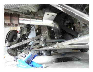
For the support bracket on the new mid-pipe you will not be able to use it with factory muffler unless some kind of modification can be done, like a custom rod bracket from the factory muffler to the mid-pipe support bracket. Note that it's not necessary to use the support bracket, you will notice that the mid-pipe is very solid even if the support bracket is not connected to the muffler.
