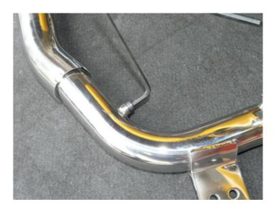
**Step 6- For 2.7L and 3.2L Owner's only**, since that you will not be using the O2 sensor ports make sure you tighten both ports on each mid-pipe.
