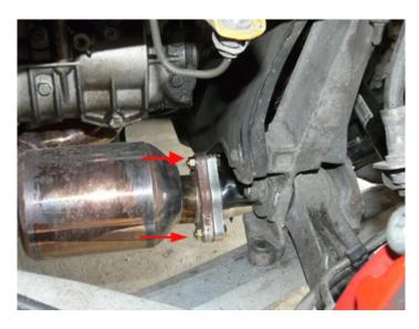
**Step 10-** Connect the double clamp to the U bend pipe, note that the U-Bend should be able to move, make sure that the mid-pipe clears the suspension, hold the mid-pipe in the correct position so that it clears equally around the suspension and tighten both the double clamp and the muffler clamp. Not that especially for the double clamps excessive force is needed to completely tighten them to avoid any exhaust leak.
