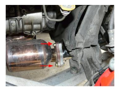
**Step 5- For 2.5L Owner's Only** all others proceed to Step 5a. Remove the O2 sensors from the factory Mid-Pipes and install them on your New NHP Mid-Pipes, it is important that you respect the position of the O2 sensors.
