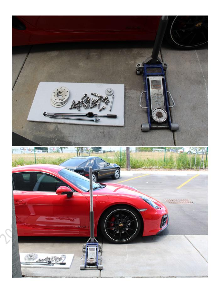
**Step 1-** Slightly loosen the wheel bolts prior to lifting the car, now raise the car and remove one wheel bolt and install the wheel guide, now remove all remaining wheel bolts.
