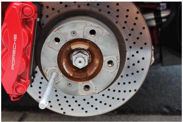
**Step 3-** Apply a light coat, again a very thin coat of wheel bearing grease or the equivalent, anti-seize compound will also work. Apply on the surface of the disc on the back of the wheel and around the hub and center bore of the wheel. Again I want to remind you to put a very thin coat.
