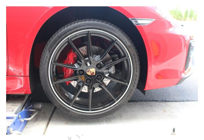
**Step 2-** Now that the wheel is off, you must clean the surface of the disc with medium grit sand paper and the hub, you must clean the back of the wheel with medium grit sand paper and the center bore of the wheel as well. All must be clean and clear from rust.
